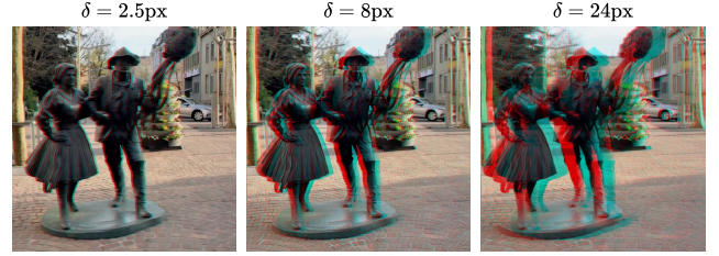
Figure 3. The strength of the stereo effect can be controlled by varying the parameter \delta that acts as a conditioning for the median disparity of the generated video (see Sec. 4.2).
